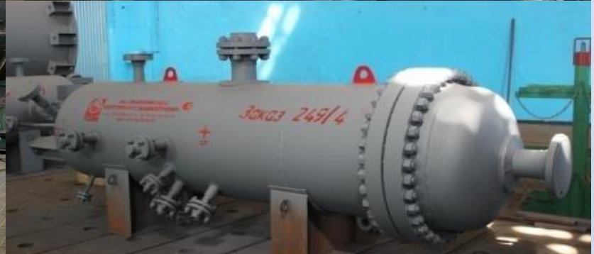
Net-shaped gas separator GS1-6,3-800-09G2S
