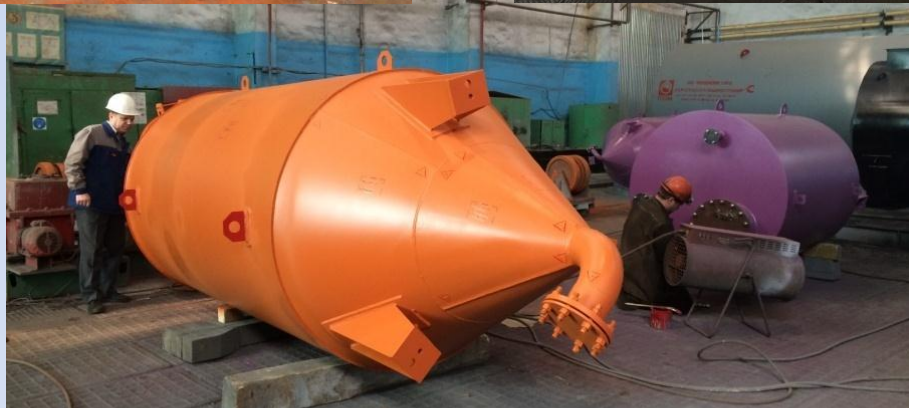
Sodium hydrate and vitriol gauging tanks
