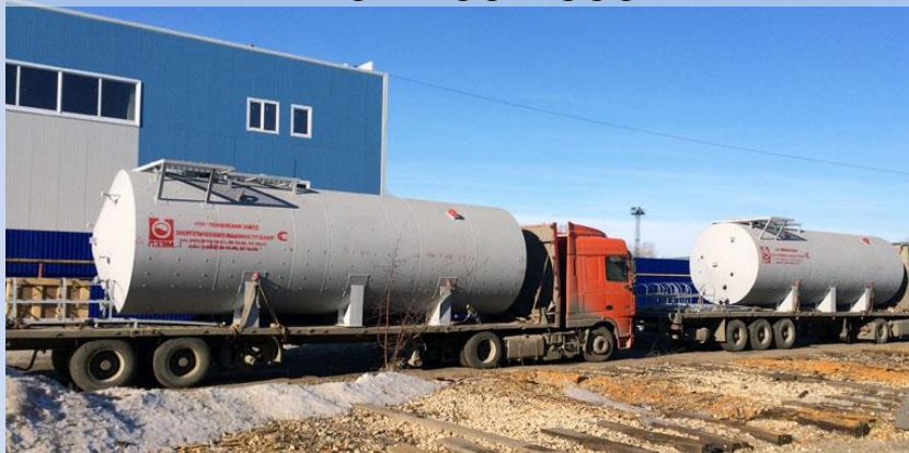
Underground vessel EP-40-2400-1000-2
