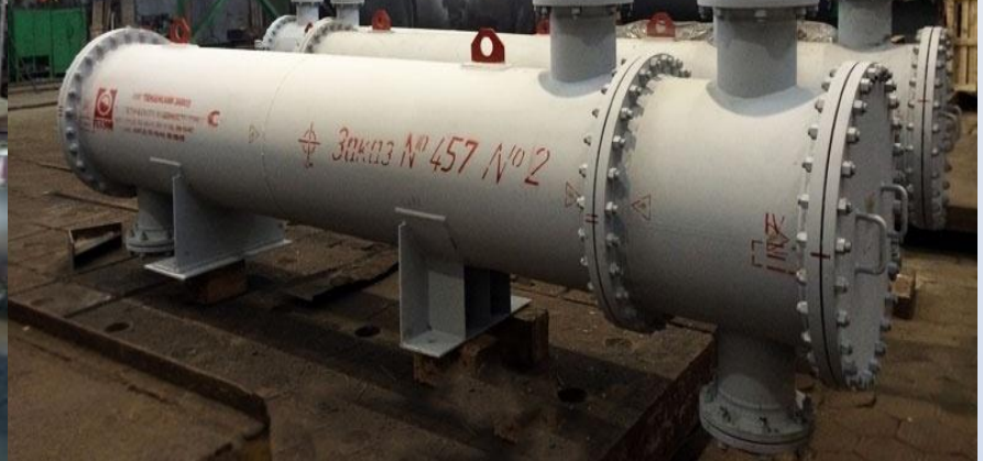
Parallel heat exchangers
