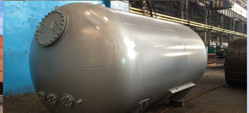
Vessel for LPG, V = 15 m 3
