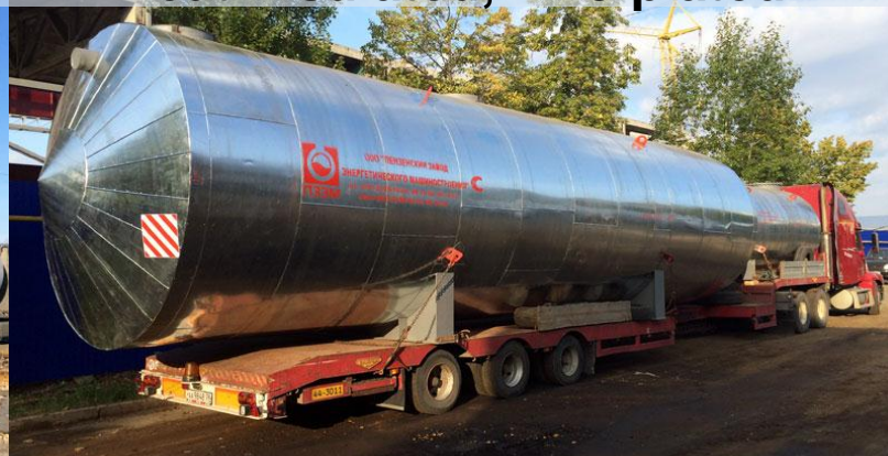
Underground vessel EP-1006 heat-insulated, zinc-plated
