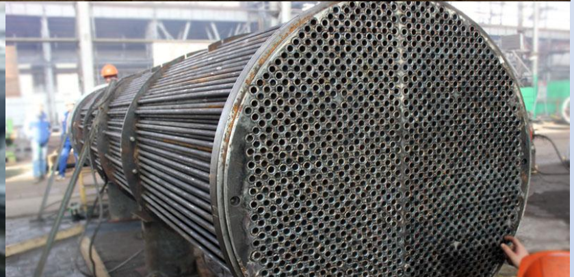
Heat exchanger 1200-TP-1,6-M1206-2-U
