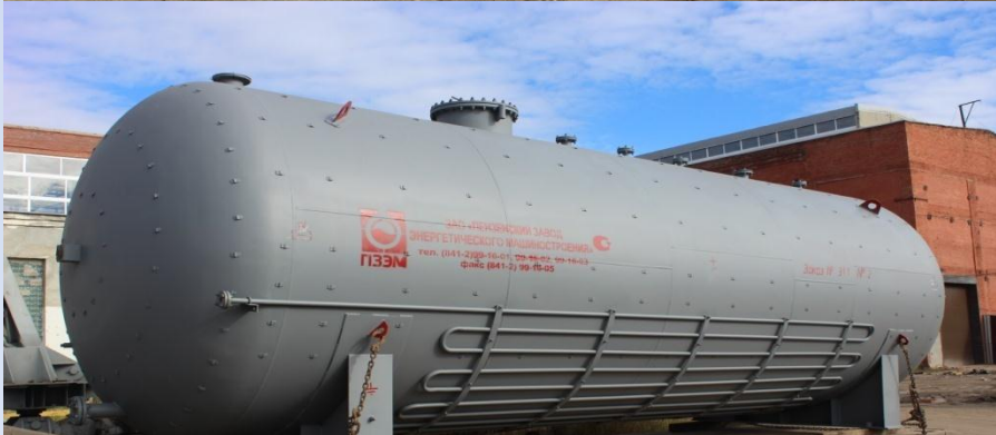
Bulk-capacity vessels handling the pressure, V = 60 m 3 , with heat-start
