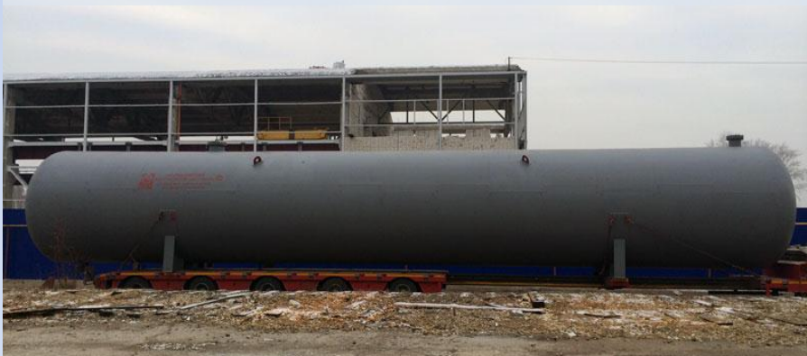
Buffer tank BS-200, V = 200 m 3
